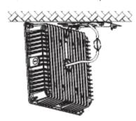
5. Install the fixture by fastening the screws on both sides of the fixture.
