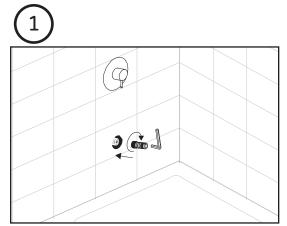
Add plumber's tape to threaded end and attach inlet nipple (1) into plumbing. Tighten using allen wrench (4) included.
