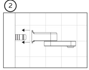
Slide spout body (3) onto nipple (1) to desired position.
