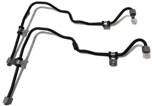
ZISTAPLEX - 8 X1 MM, Before and after a 600h corrosion test.
