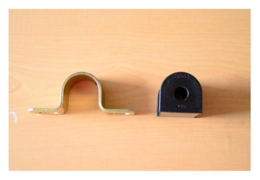
To begin, I unbolted both mounting brackets for the rear bar after pulling the rear of the car up on ramps. No matter how you elevate the car you need to be even side-to-side to unload the sway bar to eliminate any force that might be applied to the mounting bushings. There is no
