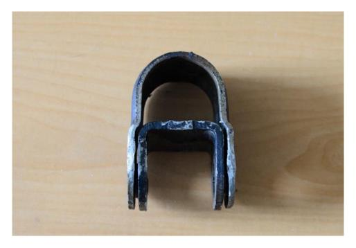
Once unbolted, twist the bracket/bushing assembly around so that the open end of the "U" is pointing down. Tap a flat-bladed screwdriver into the joint between the two pieces. By twisting the blade you can pop the bracket apart and remove it from the bar assembly.
