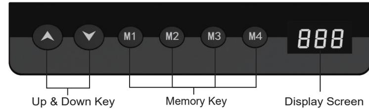
The whole handset surface is a button panel. If there is no button pressed within 30 seconds, the screen is locked and M1/M2/M3/M4 keys are locked correspondingly. To activate the display, press the Up or Down key first. The display can be used when the display screen lights up.
