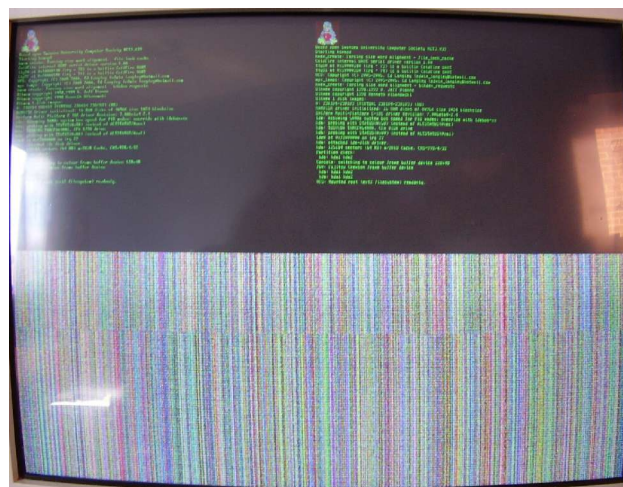
Illustration 20 An 8 bit console, with a layer width of half the value required, resulting in tiling of the layer
