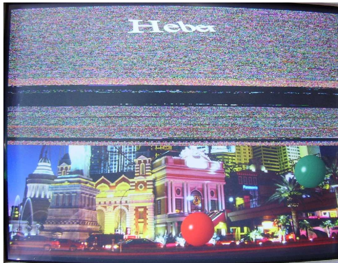
Illustration 7 The Heber Video demo halted with code downloaded; notice the black section in the middle of the code, that is the empty bss section. Also the Heber logo can be seen, this is displayed on a different layer and so isn't overwritten in video memory by the uClinux kernel
