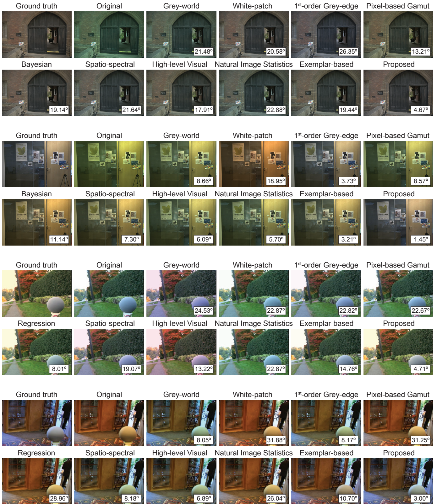
Figure 5: Some example images corrected using the estimated illuminant from various methods. The angular error is shown on the bottom right corner. Test images are corrected based on following 10 methods: Grey-world [6], White-patch [8], 1 st -order Grey-edge [10], Pixel-based Gamut [26], Bayesian [30], Spatio-spectral [32], Natural Image Statistics [22], Exemplar-based [36], and our method. For the existing methods, the results reported in [49] are directly used.
