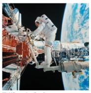
World Perspectives/Getty Images Astronauts use tools that are designed to limit forces that would impart unintended rotational motion to a satellite.
