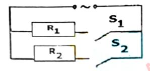
Which switches must be closed so that the heater produces the maximum possible power and minimum non-zero power?
