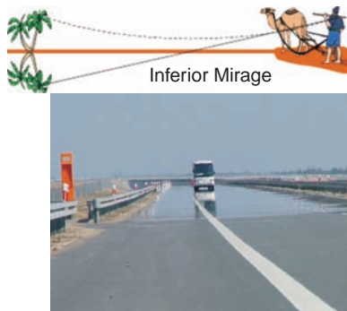
Chapter 3—Fig. 3.16 A typical mirage as seen on a hot road on a warm day. The photograph was taken by Professor Piotr Pieranski of Poznan University of Technology in Poland; used with permission from Professor Pieranski.
