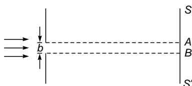
Fig. 18.1 If a plane wave is incident on an aperture, then according to geometrical optics a sharp shadow will be cast in region AB of the screen.
