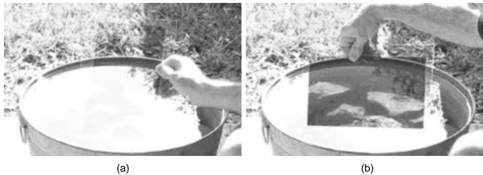
Fig. 22.11 If the sunlight is incident on the water surface at an angle close to the polarizing angle, then the reflected light will be almost polarized. (a) If the Polaroid allows the (almost polarized) reflected beam to pass through, we see the glare from the water surface. (b) The glare can be blocked by using a vertical polarizer, and one can see inside the water. Figure adapted from the website www.polarization.com/water/water.html © J. Alcoz, 2001; used with permission of Dr. Alcoz. Color photographs appear in the insert at the back of the book.
