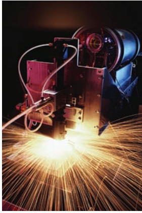
Chapter 26 A 2-kW fiber laser-mounted to a robotic system cutting mild steel. [Photograph (c) Getty Images RF]
