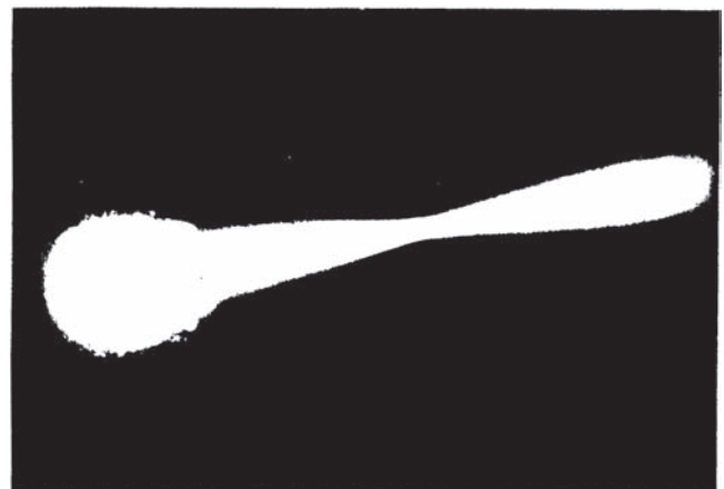
Fig. 6.5 The spherical aberration of a convex lens (photograph courtesy Dr. K. K. Gupta).
