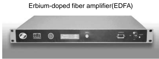
Fig. 26.10 An erbium-doped optical fiber amplifier for telecommunication application developed jointly by CGCRI, Kolkata, and NeST, Cochin. The main characteristics are as follows: 32 wavelengths can be simultaneously amplified in the wavelength region from 1532 to 1565 nm. The input power (of each channel) can be between -4 dBm ( \approx 0.4 mW) and +3 dBm ( \approx 2 mW), and the output power is always 18 dBm ( \approx 63 mW) with a gain flatness of \pm 0.5 dB [Photo courtesy Dr. Shyamal Bhadra of CGCRI and Dr. Suresh Nair of NeST].
