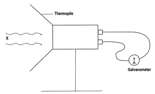
X is a radiation entering the thermopile. If the galvanometer needle shows a deflection,
