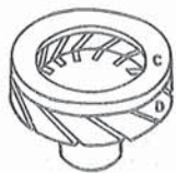
Fig. 9.6 (b) Contrate (segmented) contact
