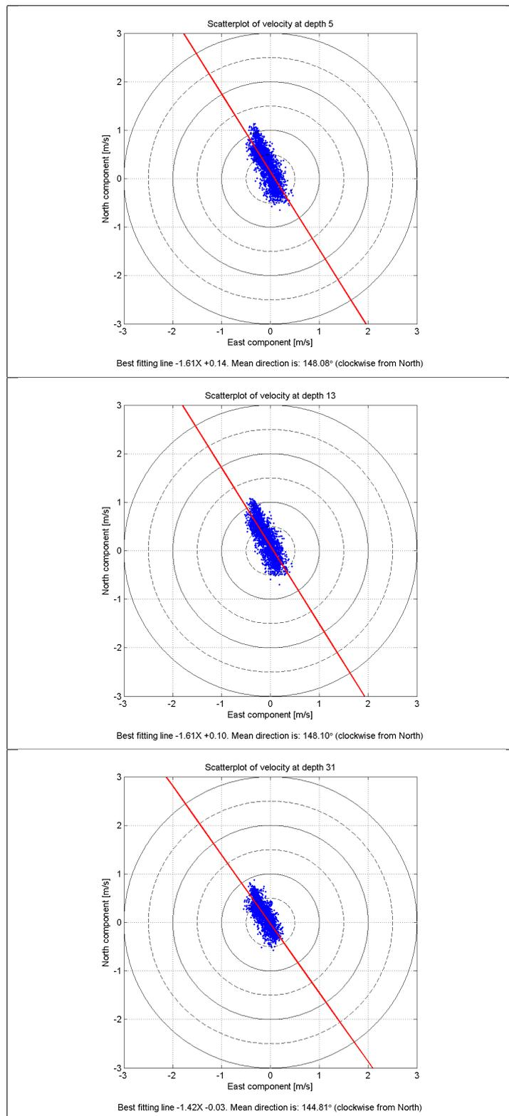
Figure 5: Scatter plot of measured velocity in North and East directions. Red line indicates best fitting mean direction
