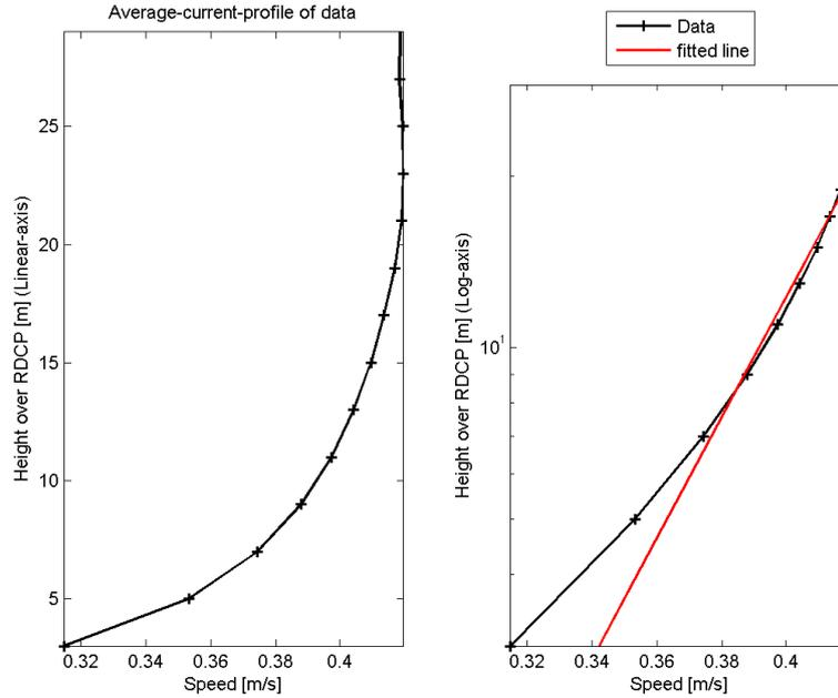
Figure 4: Average current profile in linear and logarithmic depth-axis. The red line gives the best fit to cells 3-9
