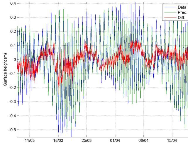
Figure 13: Time series of surface variation measured, predicted and difference.
