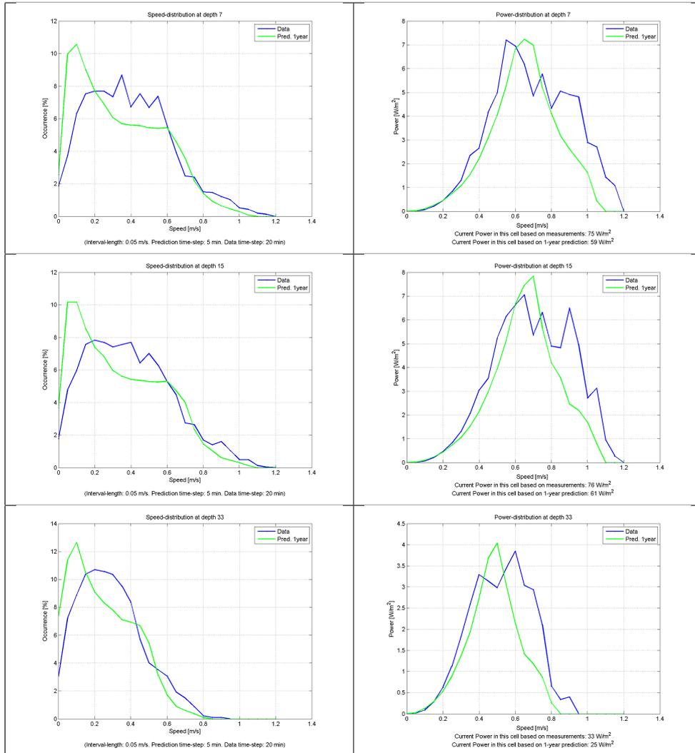
Figure 11: Distribution of measured and predicted current speed to the left, and distribution of measured and predicted power as a function of current speed
