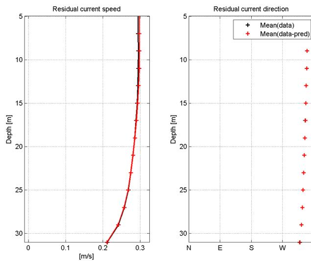
Figure 8: Profile of residual current
