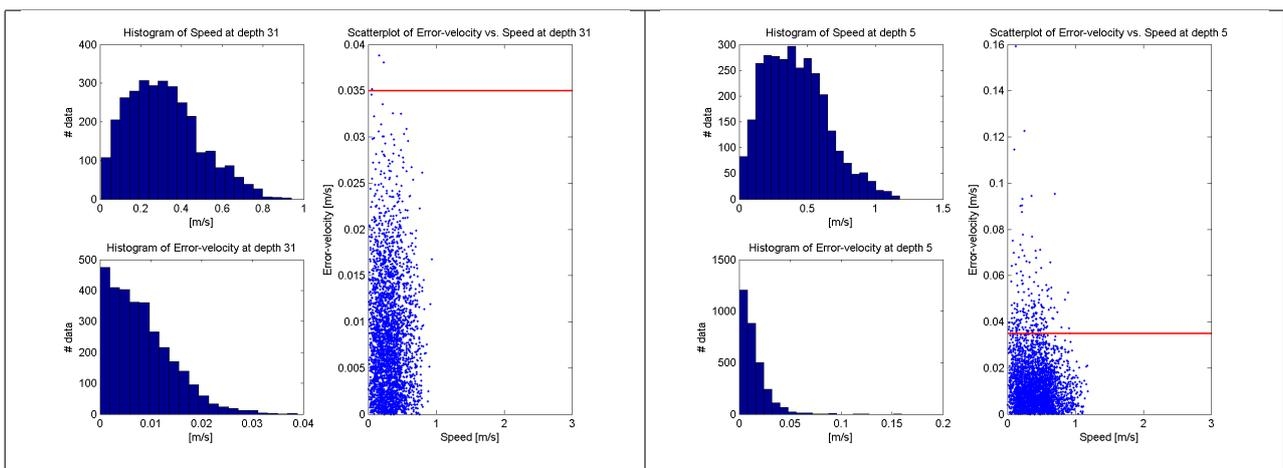
Figure 2: Scatter plot of error-velocity. The plot to the left is from the cell closest to the instrument (range 3 m), and the plot to the right is from the last valid cell (range 31 m). Red line indicates flagging threshold
