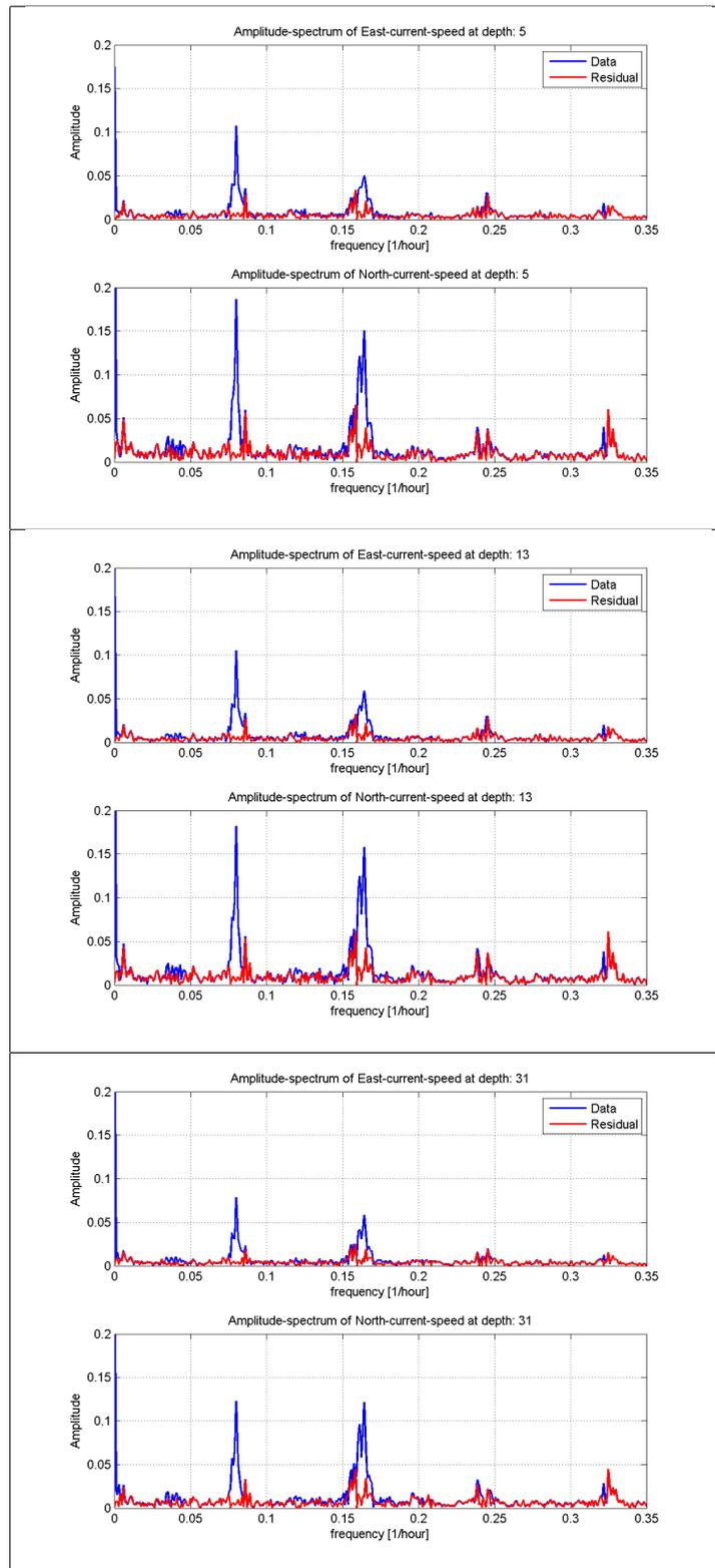
Figure 9: Amplitude spectrum at the uppermost cell (top-plot), the cell with strongest tidal current (middle-plot) and the lowermost cell (lowest-plot)
