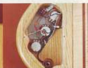
Circuit shielded by steel plate.
