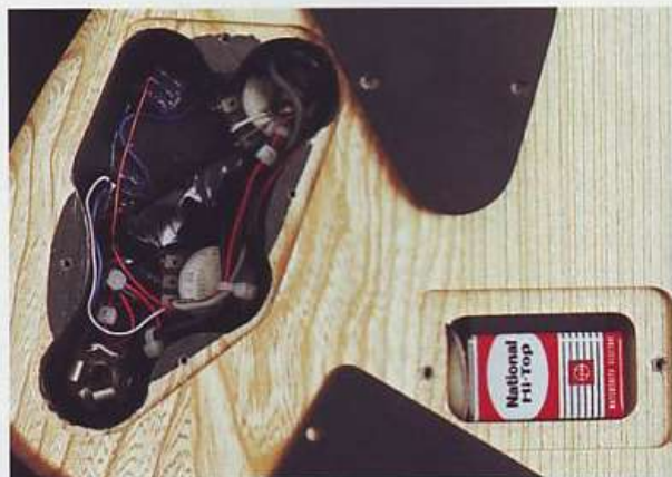
Booster Circuit powered by 9 volt battery for a year.
