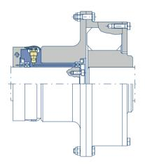
ST-KB series, integrated into the inner gear of a gear coupling
