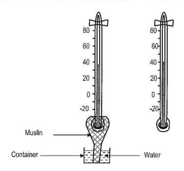
The temperature reading on the wet bulb thermometer is 35°C while that of the dry bulb is 40°C. What is the relative humidity of the air?
