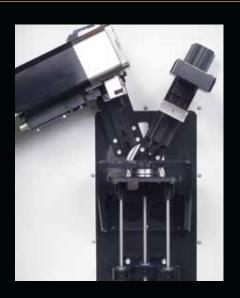
The AXRD Theta-Theta has been designed to handle larger samples or accommodate situations in which more room is needed for experimental stages, such as temperature stages or pressure cells. The flex-stage option makes mounting large samples easy, while the fully integrated cooling system keeps facility requirements to a minimum.
