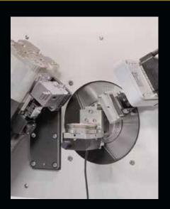
The AXRD Benchtop offers all the features of the most sophisticated powder diffractometer at a fraction of the size and cost. With an achievable FWHM peak resolution of < 0.04° 2 $\theta$  and an angular accuracy of <  $\pm$  0.02°  $\Delta$ 2 $\theta$  over the full angular range, the AXRD Benchtop is capable of producing high-quality results without occupying the space of a traditional diffractometer.
