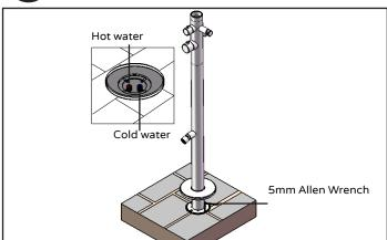
Insert bottom shower pipe (2) to the mounting base (10). Connect bottom flange to mounting base (10) with the four 5mm screws (6), then push down the bottom escutcheon.
