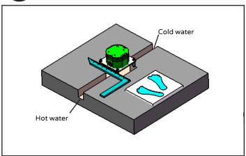
Confirm position for the mounting base (10) and standing place. Suggested distance between them is 30". Dig hole based on the mounting base (10) size.
