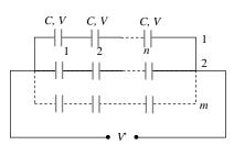
Suppose *m* rows of given capacitors are connected in parallel and each row contains *n* capacitors then potential difference across each capacitor  $V = \frac{V'}{n}$  and equivalent capacitance of network  $C' = \frac{mC}{n}$  on putting the values we get n = 4 and m = 8 $\therefore$  Total capacitors  $= n \times m = 4 \times 8 = 32$
