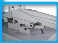
Push the handle, fast moving to open the vise
