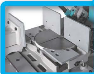
Push the handle, fast moving to open the vise
