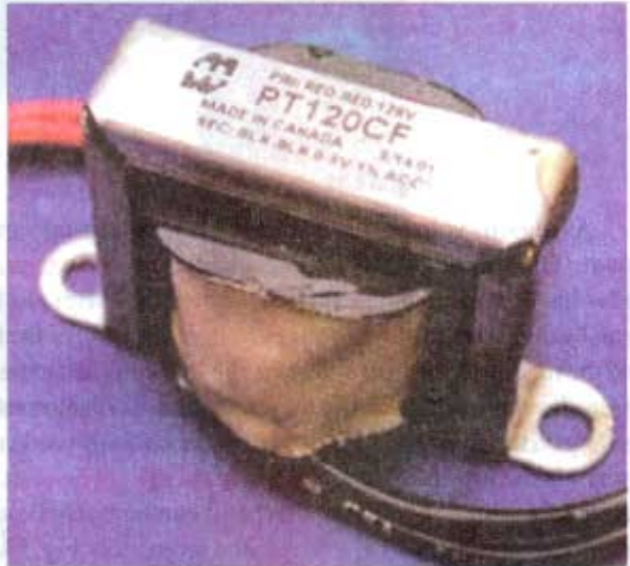
Small Potential transformer
