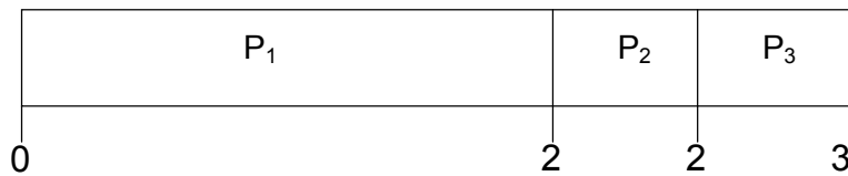
Figure 14.3 Gantt chart showing execution of processes in the order P 1 , P 2 , P 3
