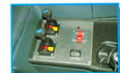
3 lock tail door trip Top and side swing taildoor
