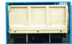
3 lock tail door trip Top and side swing taildoor
