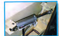
Double acting air ram actuator
