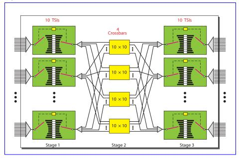
b. We can see the inefficiency in the first solution. Since the slots are separated in time, only one of the switches at the middle stage is active at each moment. This means that, instead of 4 crossbars, we could have used only one with the same result. Figure 8.5 shows the new design. In this case we still need 200 memory locations but only 100 crosspoints.
