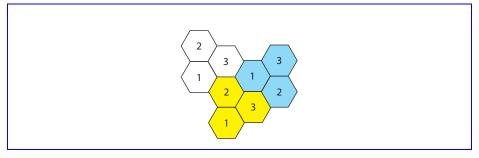
17. *In AMPS*, there are two separate bands for each direction in communication. In each band, we have 416 analog channels. Out of this number, 21 channels are reserved for control. With a reuse factor of 7, the maximum number of simultaneous calls in each cell is
