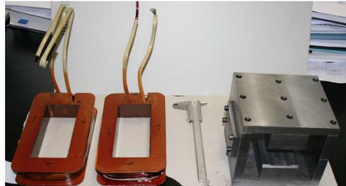
Fig. 4. Coils and iron ready to be assembled to form the magnetic part of the spectrometer
