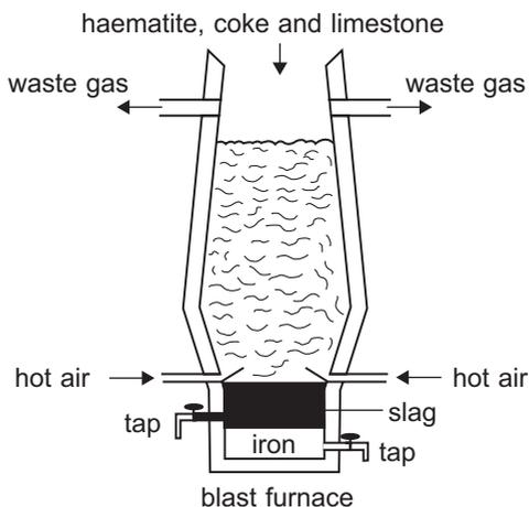
1. Coke is oxidised by oxygen in the hot air in an exothermic reaction.
