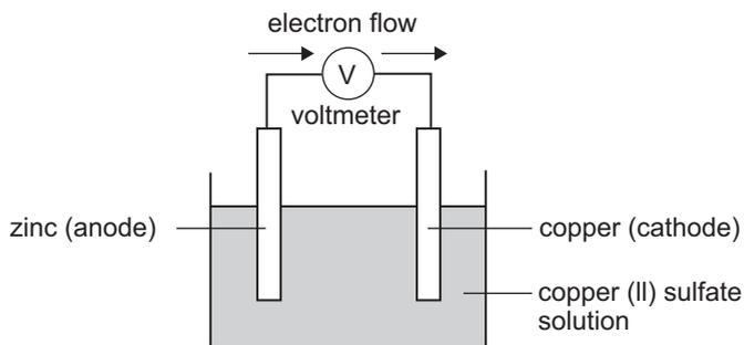
The zinc anode gradually loses mass as zinc atoms get oxidised while the copper cathode gains mass as  $\text{Cu}^{2+}$  ions are reduced and deposited. The overall equation of the reaction is obtained by adding the half-equations.
