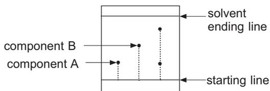
The identity of a component in the mixture can be deduced by comparing the  $R_f$  value obtained in the chromatogram with existing  $R_f$  values of known substances.
