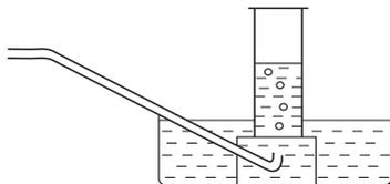
2. Downward delivery: Used to collect gases which are denser than air, such as carbon dioxide, hydrogen chloride and chlorine.
