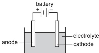
The battery provides a source of electricity for reactions to occur. During the process, electrons flow from the positive terminal to the negative terminal of the battery.
