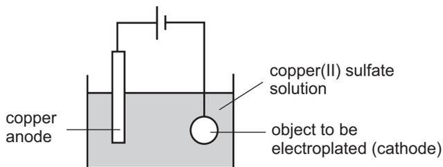
Copper metal acts as the anode as it is used to plate the object. The electrolyte used is a salt solution of its salt (copper(II) sulfate solution) and the object to be plated acts as the cathode.
