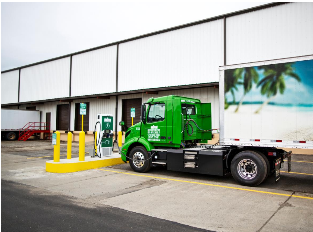
CAPTION: To support the charging of its battery-electric fleet, Manhattan Beer Distributors has installed three Level 3 DC fast chargers at its Bronx facility that can fully recharge its Volvo VNR Electric trucks up to 80 percent in 70 minutes.
