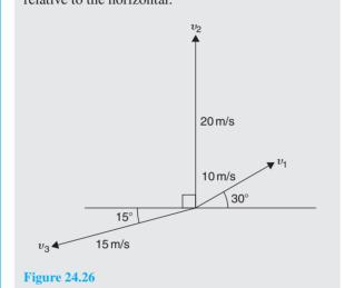
The horizontal component of the 10 m/s velocity =  $10\cos 30^{\circ} = 8.660 \,\text{m/s}$ ,
