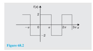
The square wave shown in Fig. 68.2 is an odd function since it is symmetrical about the origin.
