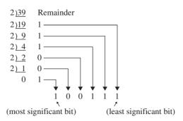
The result is obtained by writing the top digit of the remainder as the least significant bit, (a bit is a **b**inary digit and the least significant bit is the one on the right). The bottom bit of the remainder is the most significant bit, i.e. the bit on the left.
