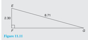
With reference to  $\angle G$ , the two sides of the triangle given are the opposite side EF and the hypotenuse EG; hence, sine is used,
