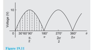
One cycle of the output voltage is completed in  $\pi$  radians or 180°. The base is divided into 6 intervals, each of width 30°. The mid-ordinate of each interval will lie at 15°, 45°, 75°, etc.
