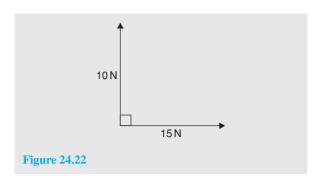
The horizontal component of the 15 N force is  $15\cos 0^{\circ}$ and the horizontal component of the 10N force is 10 cos 90°
