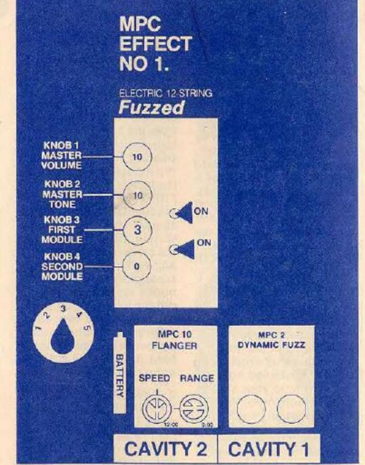
module in cavity No. 2 closest to battery. Set the speed thumb knob on the module at 12:00 as shown. Set the range thumb knob on the module at 9:00. Play full back up or rhythm type chords.
