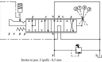
Stroke to pos. 2 (pul) - 5,5 mm "High force mode" Stroke to pos. 3 (push) - 5,5 + 5 mm "High speed mode"
