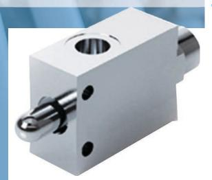
Push-to-stop valves are used to block oil passage in a hydraulic circuit (normally opened valve). The valve closes by mechanically pushing the spool.
