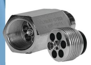
Our VPC Series hose burst valves allow free flow in both directions under normal working conditions, however, in the situation of a surge flow from 'B' to 'A' due to hose failure the valve immediately stops the flow. The burst flow can be set by increasing or decreasing dimension 'S' to be verified during final testing of the machine.
