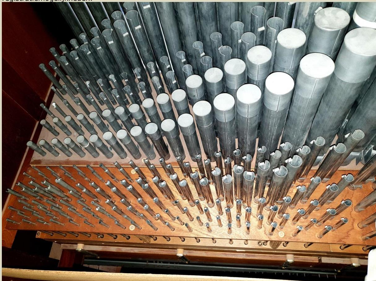
The pipework is made of different tin/lead alloys that vary between 30 and 70%. Besides metal pipes there are also pipes made of (mahogany) wood. The organ is always well maintained and in 2019 organ builder Pels & Van Leeuwen carried out a complete re-voicing. The Octaaf 2' from the Mixtuur was made independently usable by means of a pre-register; this provides more registration options.
