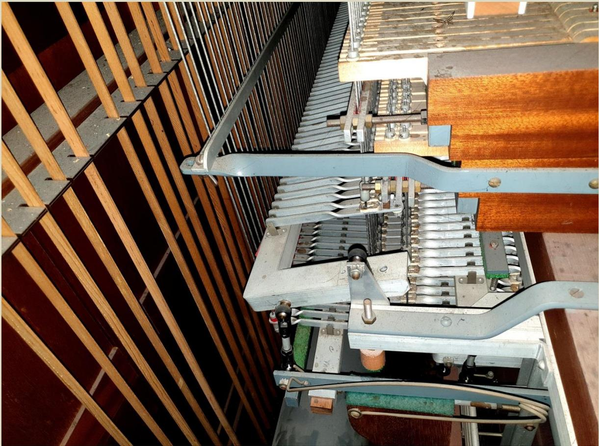
The key-action is mechanical. The trackers are made of wood and the ends are finished with linen to prevent splitting of the wood. The trackers wires are made of aluminium. The roller boards are made of wood and aluminium.
