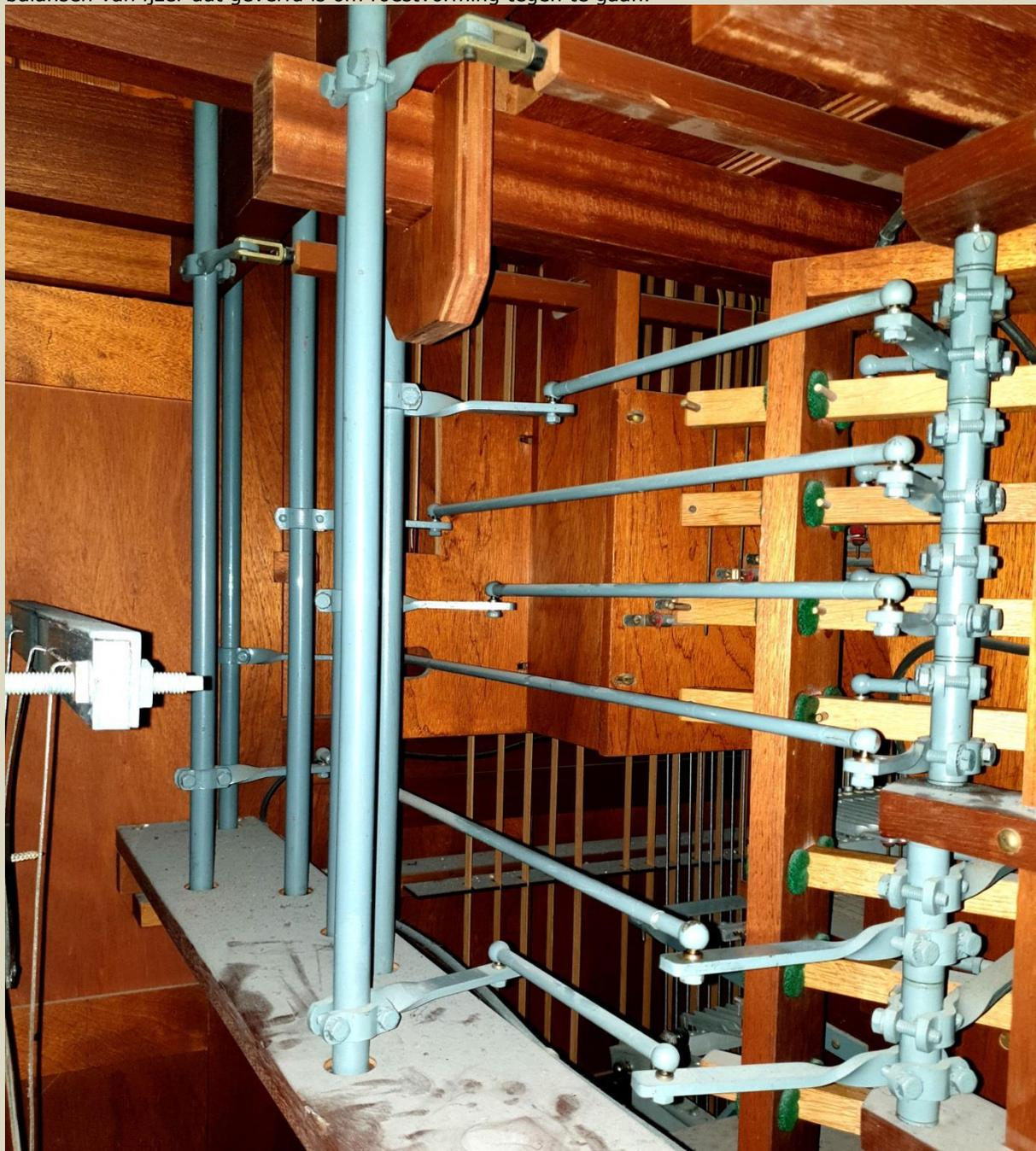
The stop action is mechanical and constructed from wood and metal. The stop knobs are situated on panels at both sides of the keyboards. The rods are made of oak, the rollers from metal upon the arms are fixed. The metal parts are painted to prevent rust.
