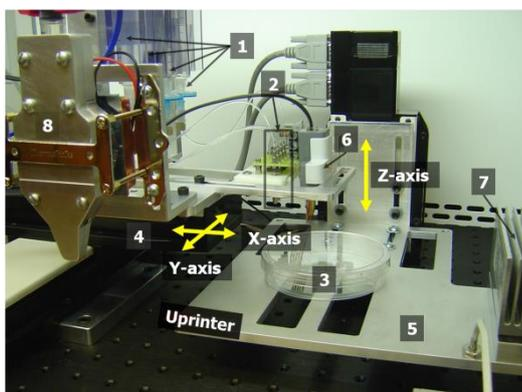
**Figure 3** Picture of the modular cell printing platform shown with [1] fluid cartridges for cells and hydrogel precursors; [2] a dispenser array; [3] target substrate; [4] X-Y stage; [5] vertical stage; [6] range finder; [7] vertical stage heater/cooler; [8] optional independent heating/cooling unit for the dispenser.
