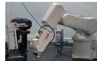
ABOVE: Robotics handling system for orienting diamonds before cutting
