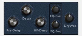
The reverb module provides a source of artificial reverberation in Odin 2. This module is sourced from Zita-rev1. The reverb additionally features a built in equalizer with a rather large Q, to further shape the reverb to your hearts desire.
