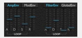
The **Amp Envelope** is hardwired to control the volume curve of the voice. This effect is not applied in the actual Amplifier module, but after the Distortion section (see the routing graphic in Section 1.5). Note that the Amp Envelope can still be used as a freely assignable modulation source in the modulation matrix. This Envelope is calculated for each voice independently.
