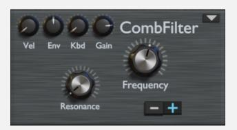
A comb filter is essentially a tuned delay module. The input signal fed into a delay-line, which echos the sound back after a set amount of time. The delay time is the inverse of the filter frequency:
