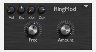
The ring modulator is an oscillator disguised as a filter. The function of this module is to multiply the input signal with an internal sine-oscillator. This is formerly known as amplitude modulation.
