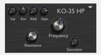
Yet another virtual analog emulation of one of the legendary analog filters of the past. This filter comes in a lowpass and highpass variant. Cranking up the resonance on these filters reveals a dirty, aggressive sound. Note that while the filters are named KRG-35, their slope is 12dB/Oct.
