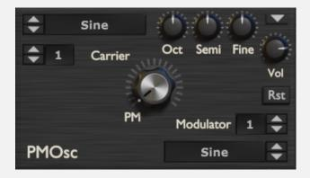
PM or Phase Modulation, is closely related to FM or Frequency Modulation. Like the FM Osc, it features a modulator and a carrier oscillator, but this time the modulator
