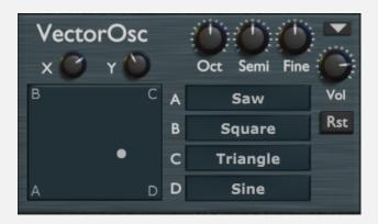
The Vector Osc gives even more options for evolving sounds than the Wavetable Osc. Four freely definable waves can be interpolated in a very intuitive graphic way via an XY-pad.
