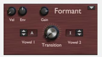
The Formant Filter tries to emulate vowels as they are produced in human speech. A tone is perceived as a vowel if two characteristic frequencies are dominant. These are called formants. The Formant Filter emulates this by using a combination of two resonator filters, which increase the frequencies around the two formants.
