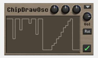
The ChipDraw Osc lets you draw a custom ChipDraw waveform. It resembles the capabilities of the "custom waveform" on an Nintendo Entertainment System (NES) sound system. The waveform consists of 32 steps in horizontal direction, which can be offset to 16 values (4Bit) in vertical direction.
