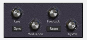
A Flanger is a modulated comb filter. The signal is fed into a delay line and mixed with the input signal after a small echo. The timing of this effect is modulated by an internal Low Frequency Oscillator (LFO). Additionally, the output of the delay line can be fed in again via the Feedback parameter, to allow for a continuous stream of echoes. The delay times for Comb Filters and Flangers is very short, usually below 50ms.
