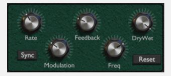
The phaser module introduces movement to the sound by applying a subtle "windy" character. The internal structure consists of a series of allpass filters: These filters do not alter the amplitude like the filters from Chapter 3, but only shifts the phase of some frequencies. By adding the phase-shifted signal back onto the original signal, some of
