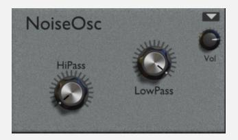
The Noise Osc provides a source of noise in Odin 2. The initial noise generation produces white noise. The noise can be further preprocessed by the included lowpass and highpass filters.
