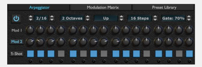
The Arpeggiator & Step Sequencer is a tool which is able to automatically play complex rhytmic sequences from a given set of input notes. Activating this module overrides the notes you're inputting into the synthesizer and generates note sequences itself.
