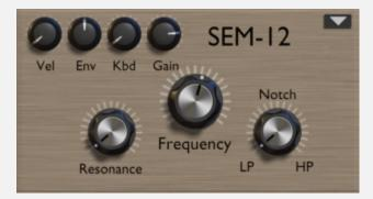
Another emulation of a classic synthesizer filter. This filter has the specialty of being able to shift between a lowpass and a highpass filter, with a notch-filter in between. The filter slope of this filter is 12dB/Oct.
