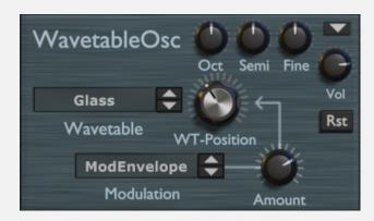
The Wavetable Osc allows you to create evolving sounds, which feature more than one waveform. Each of the 35 selectable wavetables consists of four waves itself. You can sweep through these easily by hand or with pre-setup modulation.
