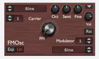
The FM Osc is a convenient way to set up Frequency Modulation, or FM. The basic idea behind FM is that you have two oscillators: The carrier and the modulator. The modulator is solely used as a modulation source for the frequency of the carrier. The carrier is the oscillator you will actually hear. While you can set up FM via the modulation matrix as well, the FM osc is the easy way to do it. The theory behind FM is very well documented in other literature, for example on Wikipedia.
