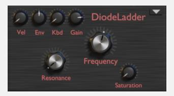
The Diode Ladder is a virtual analog emulation of another classic analog synthesizer filter. Its analog pendant was originally developed to work around a patent on the well established ladder filter. While still being 24dB/Oct, the characteristic of this filter is said to be more aggressive and wild compared to the classic ladder, especially when invoking resonance.
