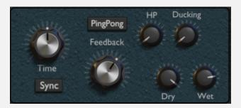
A delay is a module capable of producing an 'echo' effect: The signal is fed into a delayline, which outputs the signal again after a set amount of time again. The output of the delay line can also be fed back in, allowing a chain of attenuating echos. By controlling the delay time and feeback parameters, a wide variety of effects can be achieved. The Delay module in Odin 2 goes a step further and offers several additional features.
