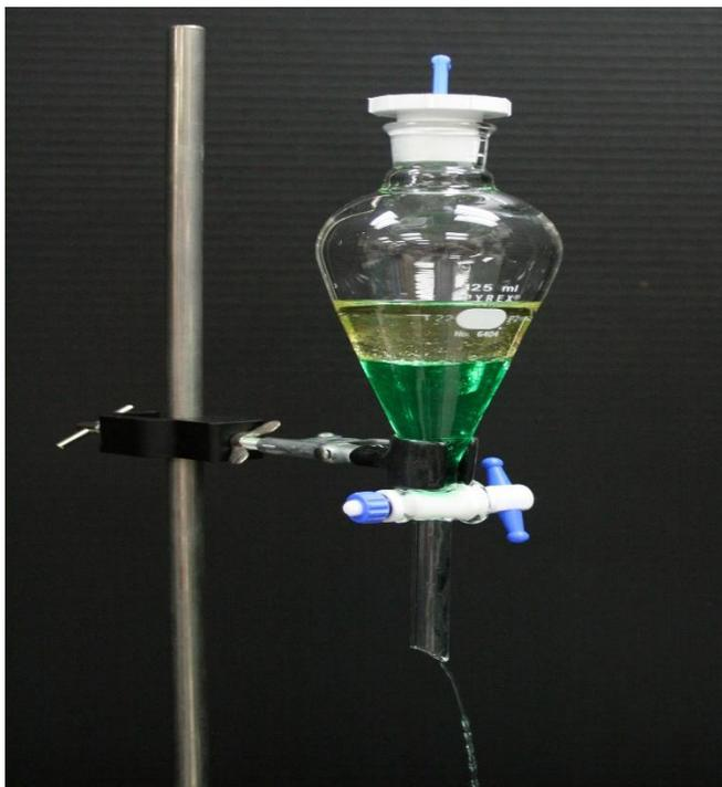
*Picture; showing an experiment on the use of separating funnel*
