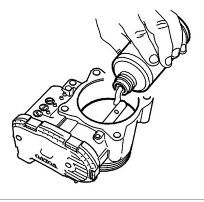
Flush the throttle unit using cleaner H on both sides of the throttle.
