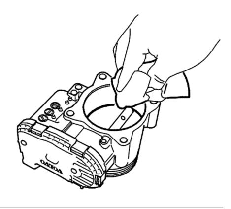
Carefully wipe the inside of the air duct clean on both sides of the throttle disc. Wipe clean the edge of the throttle disc.
