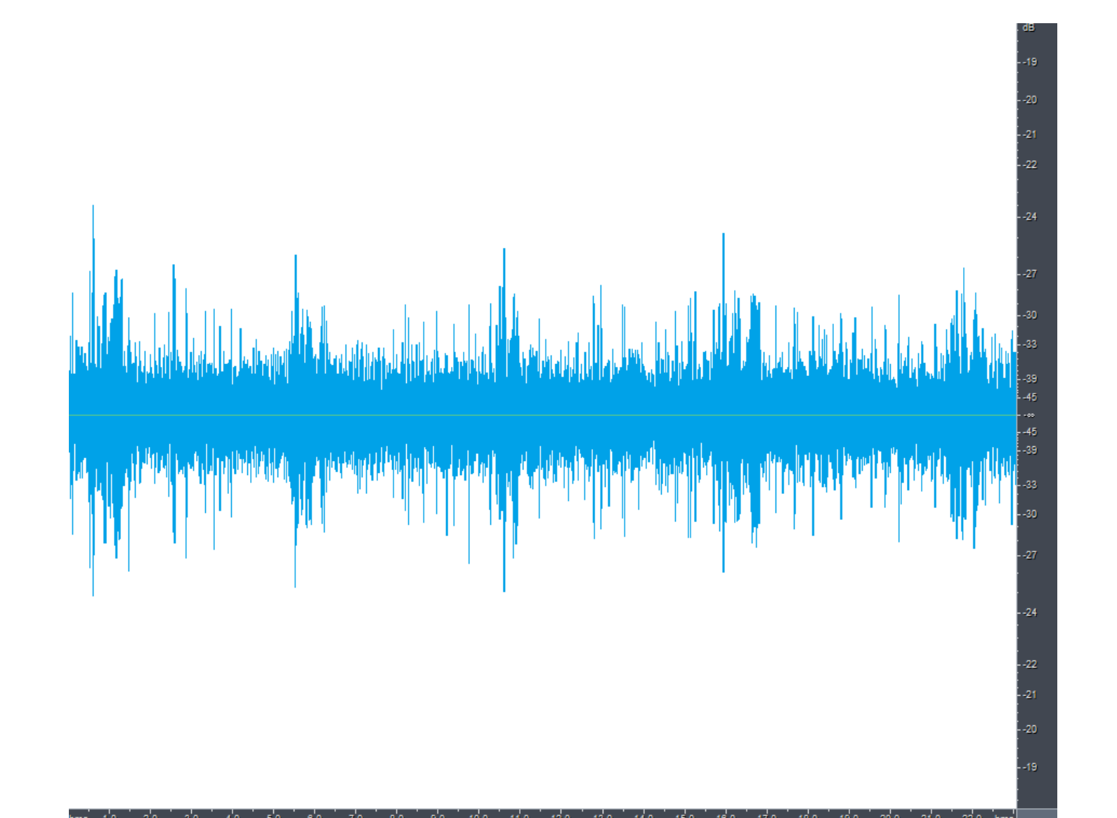
Figure 6. Time domain output of a hearing aid with a conventional ADC programmed with an adaptive directional microphone and noise reduction at 0 SNR [speech and noise at 106 dB SPL]. NU-6 words from List 1A: "laud", "boat", "pool", "nag", "limb"
