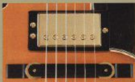
▲ Humbucking Pickup & Bridge
