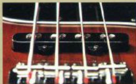
▲ 8-Pole Single-Coil Pickup
