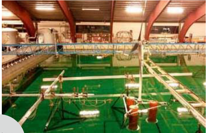
Wave tank test in the Triple Spar project
