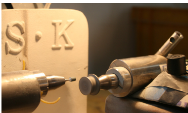
Mounted stone points dressing process
