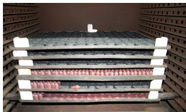
Firing furnace mounted stones
