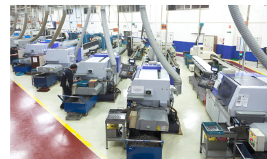
CNC Machining for Carbide burs production
