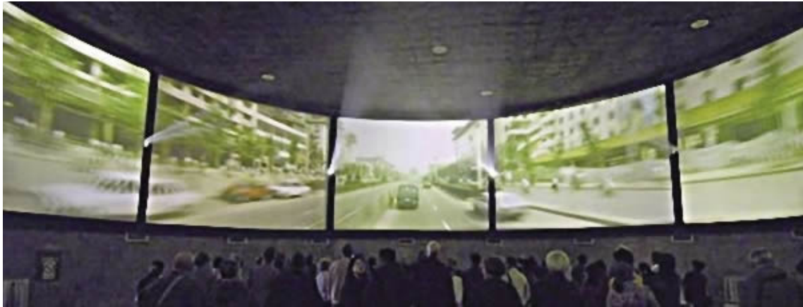
Figure 19 - Disney's Circle-Vision 360 (1955). A 9 camera/projector panoramic cinema.
