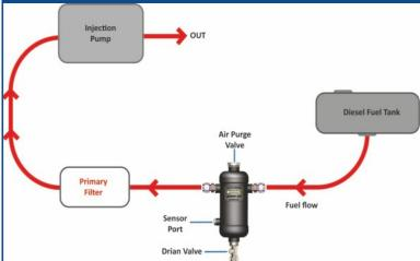
When the fuel enters the unit the baffles in the system immediately induce a swirling action, which causes water and solid contaminants to separate out of the fuel. The contaminants sink to the base of the unit where they are retained - the contaminants are simply drained and disposed of when the system is full. An optional sensor with buzzer can be supplied to indicate this.
