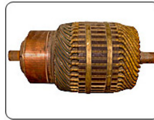
Armature with steel binding wire
