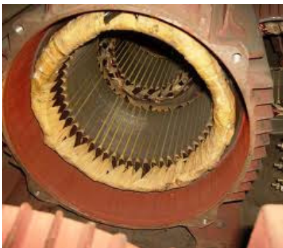
Fig.4 Stator with ribbed yoke
