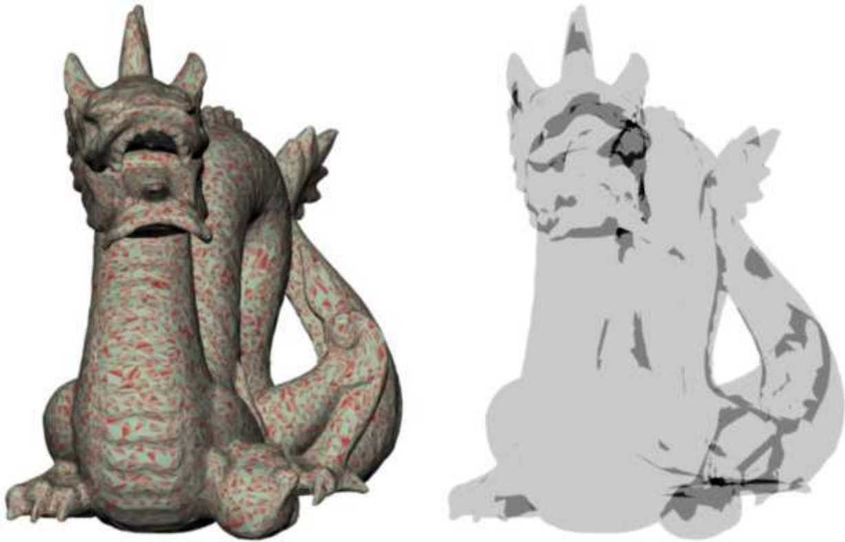
Figure 5.4: A triangle reordering study by (Sander, Nehab and Barczak, 2007). Left: The red triangles indicate areas where a vertex cache miss occurred. Right: Darker areas are portions of the frame where more overdraw occurs.
