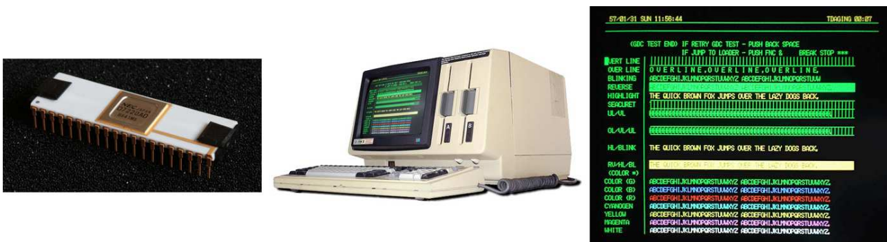
Figure 1.20: The NEC uPD7220 was used for drawing 2D points, lines and arcs to the computer's bitmap display. It was the first graphics hardware to qualify as a LSI ("Large Scale Integration") due to it containing tens of thousands of transistors in a single chip (Stengel, 2016; Bauer, 2015).
