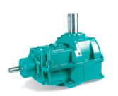
A range of single stage gearboxes is especially designed to meet the requirements for vacuum pumps drives, head-box feed pumps and centrifugal pump drives. Next to the standard arrangement with shafts in a horizontal plane, the gear unit can also operate with both shafts in a vertical plane: high speed shaft above low speed shaft. This brings the high speed shaft height more in line with shaft heights in standard IEC electric motors.
