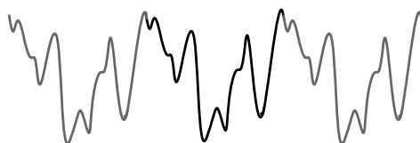
Clarinet waveform E b , 156 Hz
