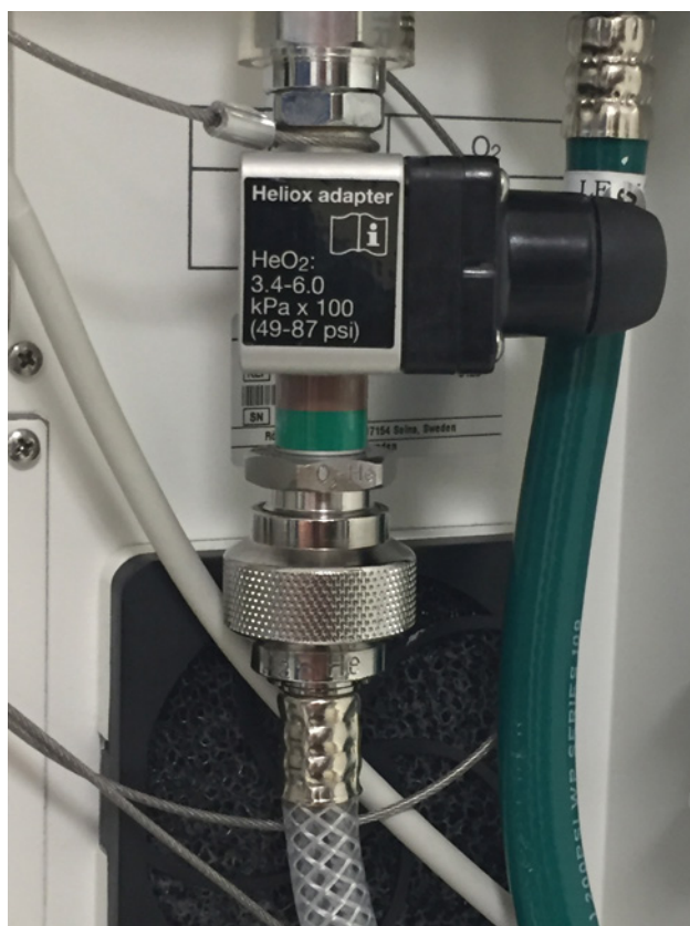
FIGURE 29-2 A special adaptor is used to connect a high-pressure hose to a heliox tank and the 50 psi air inlet on a ventilator.
