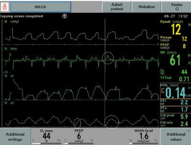
FIGURE 26-4 An example of using NAVA graphics to set the NAVA level. The lavender spike originates from the beginning of diaphragmatic contraction, indicating that the Edi trigger is appropriately set. A lavender spike that appears higher on the diaphragm signal means that trigger is set too high and the activity is not picked up until the diaphragm is partially contracted. A signal displayed on the down slope of the signal means that trigger is set too low and the ventilator is detecting diaphragmatic activity during the relaxation phase. When there is no detection of a diaphragmatic signal with a flow-triggered response the ventilator will deliver a pressure-supported breath.
