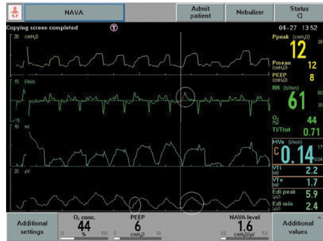
FIGURE 27-14 An example of using NAVA graphics to set the NAVA level. The lavender originates from the beginning of diaphragmatic contraction, indicating that the Edi trigger is appropriately set. If the lavender spike appears higher on the diaphragm signal, the trigger is set too high and the activity is not picked up until the diaphragm is partially contracted; conversely, if the signal is displayed on the down slope of the signal, the trigger is set too low and the ventilator is picking up activity during the relaxation phase. Note the lack of diaphragm signal with a flow-triggered response will cause the ventilator to deliver a pressure-supported breath.
