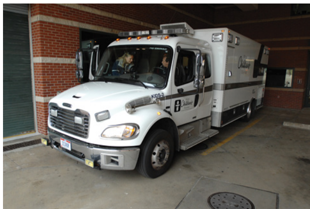
FIGURE 33-1 An example of a neonatal/pediatric specialty ground ambulance. The ambulances are equipped to be mobile ICUs.
