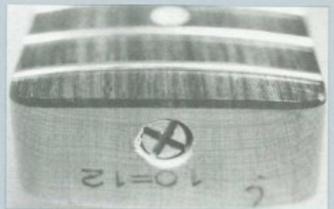
Brass pickup and control network shielding eliminates noise.
