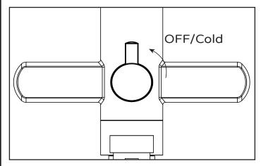
For handshower to be OFF the diverter handle should be facing up. The closer to the OFF position, the colder the water will be.
