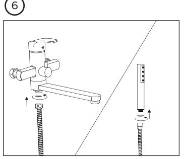
Once handshower holder is secure, insert rubber washer into both ends of hose. Connect hex head end to tub filler and tapered end to handshower. Place the tapered end of the hose into the handshower holder.
