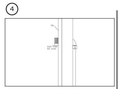
Keep the distance of the connectors 0.33-0.35 inches (8.5-9 mm) to the surface of the tile.
