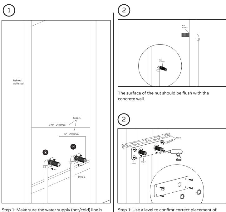
Step 1: Make sure the water supply (hot/cold) line is 6 inches (200mm) apart from the center of the Hot & Cold water supply pipes.
